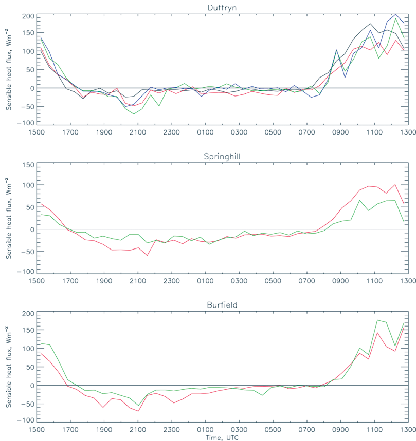
Fig. 9. Sensible heat fluxes for 9–10 Sep 2009. Lines are at the following levels: black is 2 m, red is 10 m, green is 25 m (Duffryn) and 30 m (Burfield and Springhill), and dark blue is 50 m.
