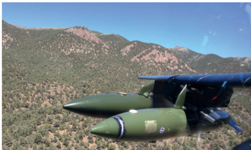
FIG. 3. Alpha Jet pods. The near pod (with unpainted ring) is the instrumented pod. Note the reflection of the pilot’s helmet in the canopy. (Photograph courtesy of R. Simone.)
