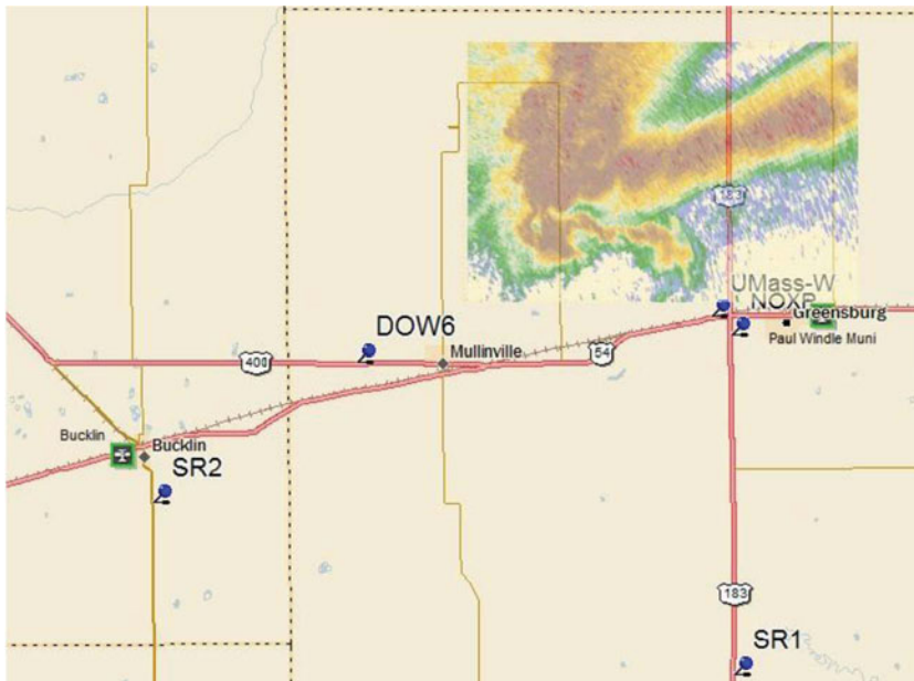
FIG. 5. Snapshot of actual deployment of various radars. Storm and mesocyclone-scale radars are deployed in real-world road and terrain conditions in Kansas on 9 Jun 2009 on a marginally tornadic supercell to establish multiple-Doppler coverage.
