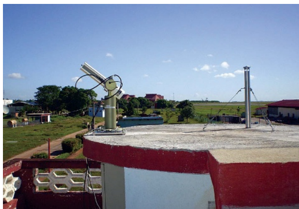
FIG. 4. (left) CIMEL sun photometer and (right) collecting nose of the impactor operated by GOAC at Camagüey, Cuba, under a joint cooperation agreement with the GOA-UVA. Sun photometer measurements are contributed by RIMA and AERONET.
