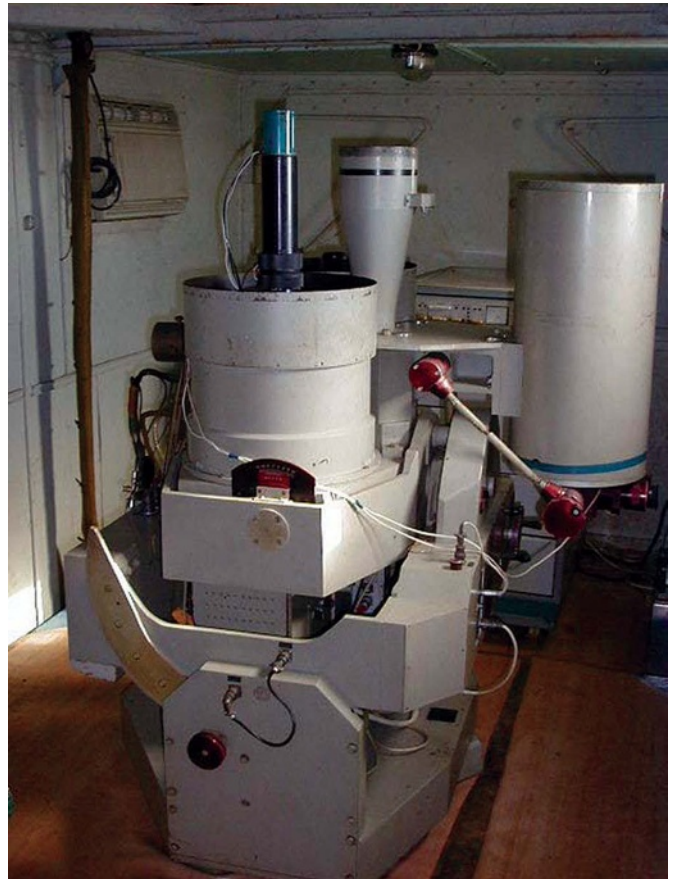
FIG. 1. Maket-2 lidar instrument installed at Camagüey in 1988.
